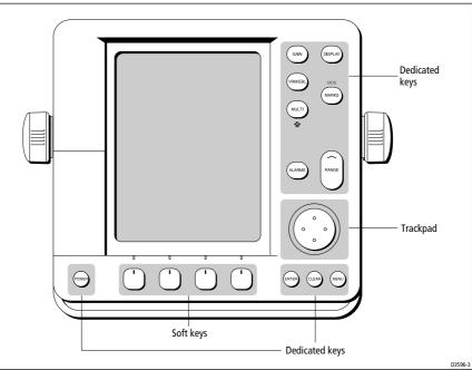
Figure 1-2: LCD Display Control Keys
